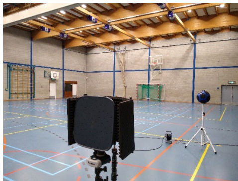
Figure 6: The measurement setup to gather a sound map of reflections in sports hall OV. On the left is the Sorama CAM iV64 acoustic camera surrounded by the shield. On the right is the omni-directional speaker.
